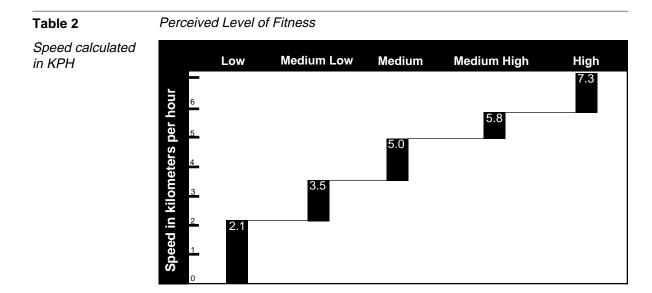
Set the speed of the treadmill based on your perceived level of fitness (low, medium, or high—see Table 1 or Table 2). The incline is preset to accommodate your level of fitness.
